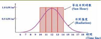
If you are getting 4 hours of direct sunlight averagely each day in a year, you can calculate it this way: 4 hours x 1,000 watts = 4,000 watts or 4 kilowatt hours (kWh). Thus this 1kW system would produce 1,460 kWh of energy per year (365 days based).
